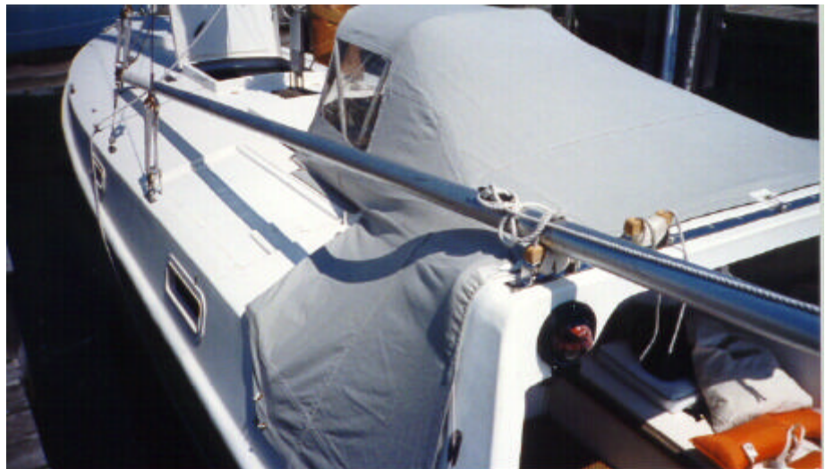
Dodger Installed Note rainproof fit... now bring on the wind and rain!
